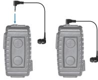
In order to be able to hear incoming signals received by the two-way radio, the PRYMEBLU Lapel Microphone must be used with an earphone. A PRYME EH-1189SC ear bud-style earphone is included with the PRYME Lapel Microphone kit.
